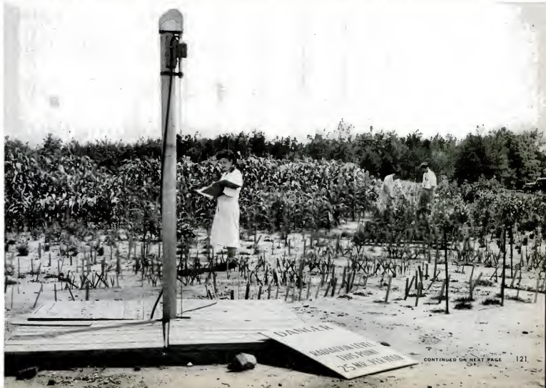
RADIOACTIVE COBALT MOVES UP AND DOWN IN A HOLLOW PIPE AT THE CENTER OF THE FIELD. WHEN WORKERS ARE PRESENT IT IS LOWERED INTO GROUND
