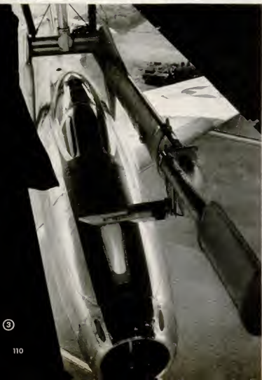
F-4 IS RAISED INTO B-36'S BOMB BAY AFTER CONTACT WITH "TRAPEZE"
