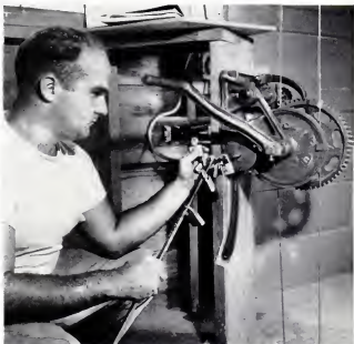
COBALT CONTROL, a winch, raises and lowers cobalt source. When it is lowered into ground, lead and earth shield fieldworkers from its radiation.
