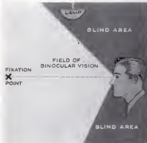
Side view of field shows how it is narrowed by cheeks and brow. The lamp is invisible, as in diagram above.
