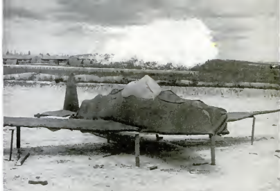
Dummy plane, made of lath and burlap, is parked a good distance from hidden hangars to decoy bombers, fool enemy observation ships. From the air, this is practically indistinguishable from a real plane.
