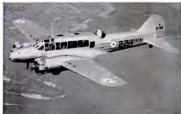
Avro Anson is for coastal reconnaissance, which is highly useful for anti-submarine work. It carries ten bombs. In case its bombs miss, it reports the presence of a sub to surface craft. A slow plane with a maximum speed of 188 m.p.h., it will help patrol Britain's shores.
