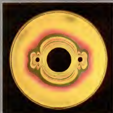
Smaller flywheels' stress patterns are analyzed by engineers who are able to predict where their full-sized prototypes are most likely to fail. A small change in the flywheel's design may completely alter the pattern.
