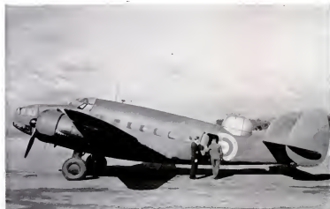
Lockheed Hudson is one of 200 American Lockheeds bought by the British. Now used largely for training, it will also be useful in war for general scouting, light bombing, submarine reconnaissance. It has a range of 1,700 miles and a maximum speed of 246 m.p.h.
