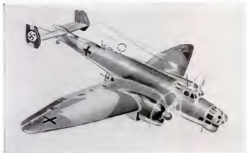
Junkers Ju. 86K is a medium bomber which, like all the models shown here, is being sold for export. Export models are slower than regular army models, whose performances are kept secret. The 86K does 250 m.p.h., is powered by either Diesel or gasoline engines.
