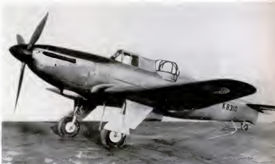
Boulton Paul Defiant is a new secret fighter which can do better than 300 m.p.h. Called a multi-seat fighter, it carries a gunner in addition to the pilot. The gunner sits in the turret behind the pilot, fires a brace of machine guns. The pilot fires guns fixed in the wings.
