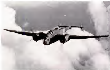
Handley Page Hampden medium bomber has a range of 1,750 miles at average cruising speed of 212 m.p.h. Most efficient medium bomber in the R.A.F., it carries a crew of three. The pilot sits in upper front cockpit. Behind him is a machine-gunner. In glass nose sits the bomber.
