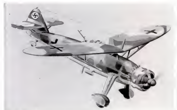
Heinkel He. 126 is a two-seat observation, which is not so good as Britain's Lysander. It has a speed of 220 m.p.h., range of 680 miles, is used for front-line reconnaissance, can lay smoke screens. Like most observation planes, the He. 126 is high-winged for better visibility.
