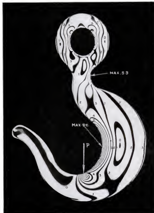
The danger points in the crane hook, paradoxically, are at the thickest part, as shown by the closely packed stress lines seen at the inside curve of the hook.
