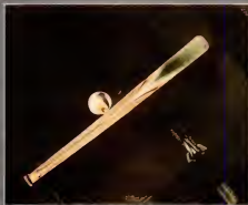
Hitting a baseball does not strain the bat when properly done ( above ). But contact too close to handle sets up extra strains, which may break the bat. The bat will also sting the batter's hands, as stress lines indicate.
