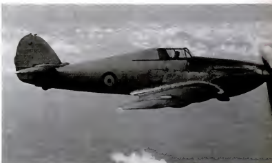
Hawker Hurricane is an interceptor with a top speed of 336 m.p.h., can stay up two hours. It can climb from the ground to 10,000 ft. in a little more than four minutes. Only new Hurricanes have the variable pitch propellers, which are important to quick-climbing planes.
