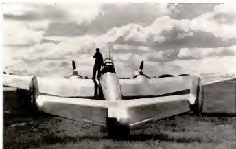
Potez 63 is also a combined bomber-fighter-scout, but a good design job. As a light bomber, it does 279 m.p.h., has a range of 800 miles. Without a bomb load, her speed is 283 m.p.h. Production is slow, however, only one plane a day coming from the factory.
