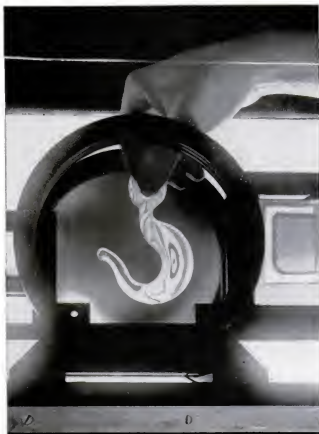
A giant crane's hook becomes a tiny transparent model. But this model with its "frozen" stress patterns tells engineers whether its massive prototype will work.
