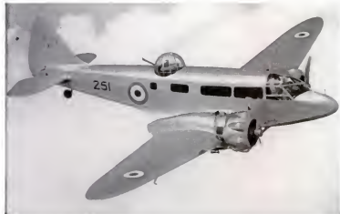
Airspeed Envoy , a light twin-engine ship, is equipped to do general scouting but its main function is to transport army and air-force personnel and valuable, quickly needed freight like radio equipment or airplane parts. Its top speed is 200 m.p.h., its range is 620 miles.
