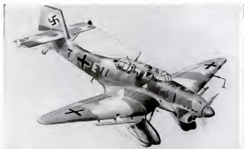
Junkers Ju. 87 is a dive bomber, a type which proved remarkably effective during the war in Spain. It picks its target high in the air, power dives on it, pulls out sharply at about 2,000 ft. to drop its load of bombs, then speeds away. Air flaps on wing front check its descent.
