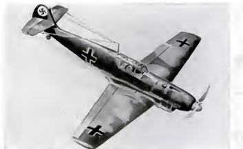
Messerschmitt 109 is Germany's most famous fighter which, even in export models, has a speed of 354 m.p.h. Cheap to manufacture, easy to produce, it is an ideal pursuit plane. Its 20-mm. gun fires shells through the propeller hub. Much like it is Germany's Heinkel He. 112.
