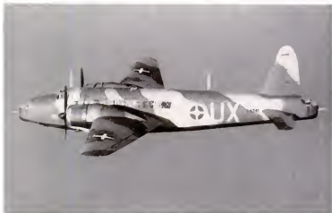
Vickers Wellington heavy bomber is Britain's biggest military land plane. When loaded, it has a range of 3,200 miles at a speed of 180 m.p.h. This ship can bombard Berlin from British air bases. The R.A.F. has about 200 Wellingtons, gets new ones at the rate of one a day.
