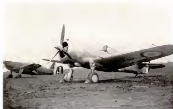
Curtiss Hawk 75A is the American pursuit plane, long standard as the P-36 in the U. S. Army, which is now buying faster fighters. Its speed is about 300 m.p.h., its range unusually long among European fighters. Curtiss-Wright has sold 209 75A's to France.
