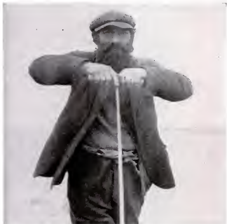
Prospector thrusts a 6-ft. "divining rod" into the ground. If the rod meets metal, particles adhere to its file-like tip. Several thrusts indicate the size of buried shell.
