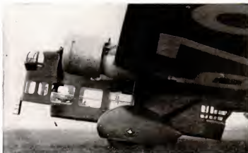
Amiot 143-M , a two-story crate, typifies the troubles of the French. Designed to do either bomber, fighter or scout duty, it is too slow for bombing and too clumsy for fighting. Its type proved to be death traps in the Spanish war. Top speed with bomb load is 189 m.p.h.
