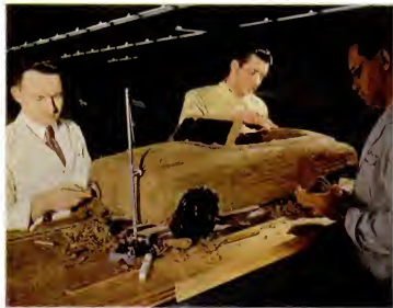
DESIGN FOR NEW CAR begins with small-scale clay model. When Studebaker management gives order for new car each of 10 designers works up his own ideas into model under general direction of Raymond Loewy. Company heads then choose best design.
