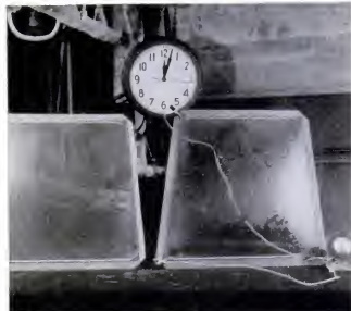
NESA-COATED WINDSHIELD clears sufficiently to permit adequate vision in less than three minutes. Clearing starts at top and bottom of glass.
