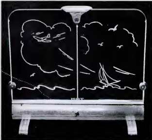
AUXILIARY HOUSEHOLD HEATER is made of two pieces of tempered glass with one Nesa-coated on inside. Glass is edge-lighted by tube in base.
