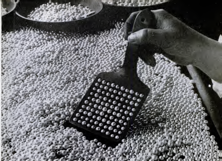
COUNTING PEARLS is speeded by sifterlike gadget shown above, with 100 pearls resting in its small holes. The pearls slip easily into the holes, then they are transferred
