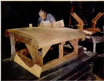
MAHOGANY MODEL of new car body is made to great accuracy. It is used to determine measurements of big dies which stamp out production line bodies and is also basis for design of body jig ( top picture, opposite page ) which holds bodies during welding.
