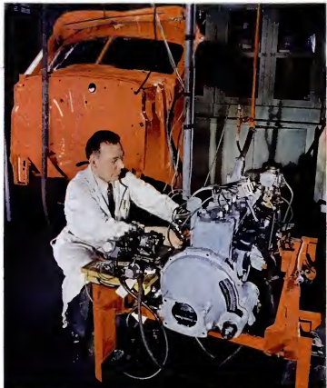
CONSTANT TESTING of parts of cars is carried out in engineering laboratory. Here technician is testing starting mechanism. In background, truck windshield wipers are on an endurance test. They worked continuously for 2,500 hours before breaking down.
