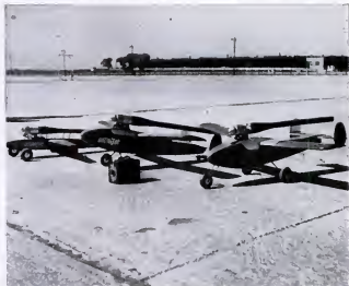
JET MODELS did not compete. "Minijet" engines weigh 16 ounces, burn gas in a true pulse-jet power unit like those used in German V-1 buzz bombs.
