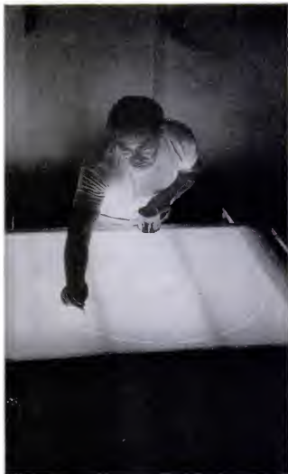
AT CADWALLADER FACTORY design is transferred onto a gelatin-coated silk screen by an exposure table. Here a workman retouches the outline.
