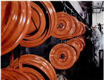
WHEELS ARE PAINTED as they move past man with spray gun. Studebaker buys its wheels from Detroit plant of Budd Company. Overhead conveyers like the one in this picture run all over plant, carry everything from whole engines to trays of tiny washers.
