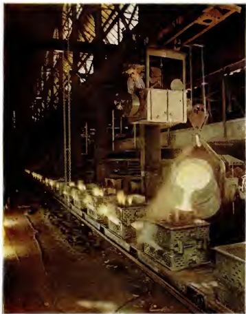
CYLINDER BLOCK MOLDS are filled with molten iron from bucket as they move on conveyer in foundry. When metal has solidified, molds are cracked open and blocks lifted out. They are then machined and fitted with pistons, camshaft and crankshaft.
