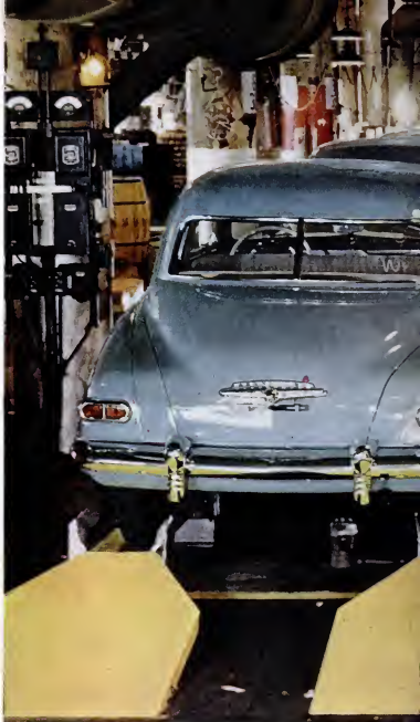
AT END OF PRODUCTION LINE shiny new Studebaker sedans, already filled with gas, oil and water are backed off under their own power. Although a new car comes off dual line every minute during nine-hour day, it takes approximately four days for body
