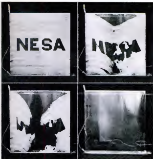
BEEWAX COATING melts completely in one minute after a 250-volt current is passed through Nesa-treated glass. The final temperature was 165° F.
