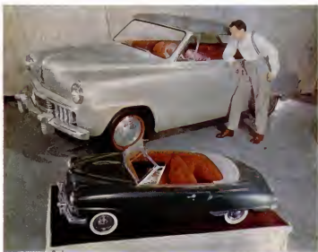
BIG AND LITTLE MODELS of convertible are shown together. Scale on plaster model ( foreground ) is one-quarter inch to one inch. Wooden model ( background ) is full size. Left door will open and close, but it has no engine or chassis and its wheels do not turn.
