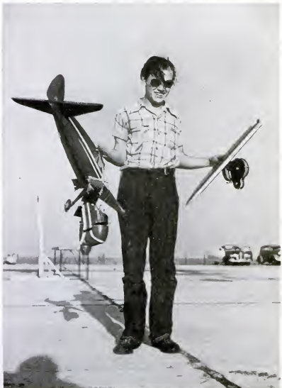
WRECKAGE of his plane is ruefully displayed by 15-year-old Ed Jackson of Deuver. It crashed on a concrete runway after the control line broke. Ruined motor cost $30, other parts about $10.
