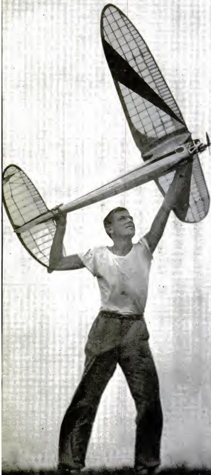
TINY JET PLANE zips through an 80-mph demonstration flight, guided by Designer Keith Goodwin. He controls plane by wires not visible in picture.
