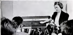
METRONOMIC READER forces children to read at a set pace without looking back. Printed on roll, story appears at slot a third of a line at a time.
