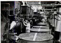
Roasting Machines With "Brains". After skillful blending by A&P experts, the coffee reaches these exclusive automatic roasters that cut off the heat the instant the roast reaches its flavor peak.
