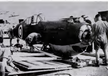
Curtiss Tomahawk is assembled at R. A. F. station in Middle East. The British would prefer long-range fighters. But till U. S. factories begin producing them Britain will have to wait.
