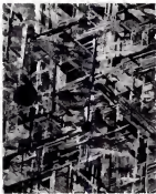
Network of lines, known as Widmanstätten figure, shows when a meteorite is polished, etched with acids. They are the result of rapid crystallization.
