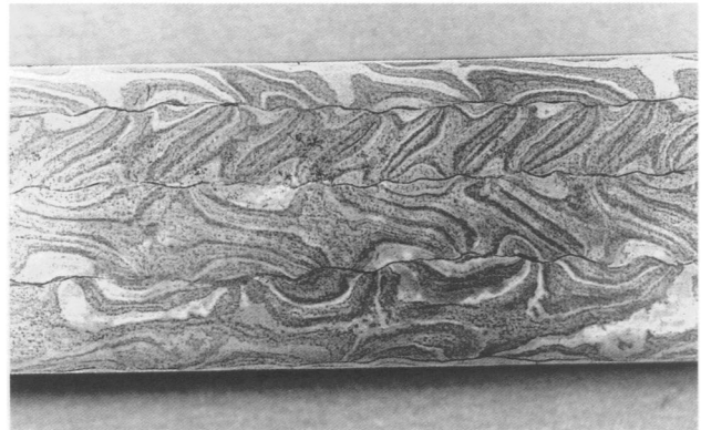
Figure 14. Detail of blade on a peidao , 17th–18th century, showing four-row huawengang and inserted edge plate. Courtesy Scott M. Rodell, Great River Taoist Center, Washington, D.C. (photo: author)
