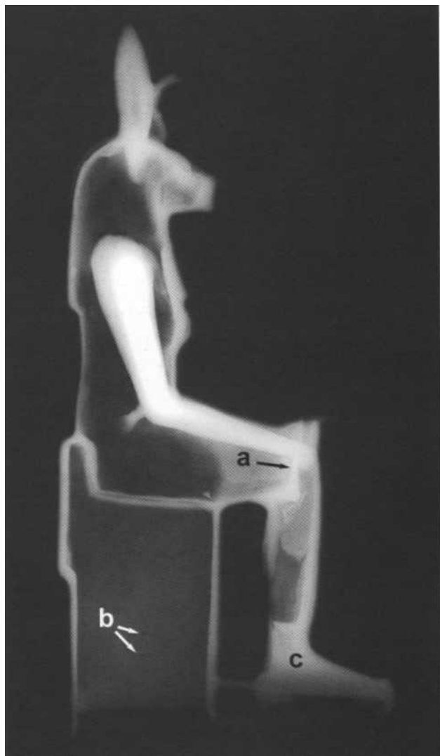
Figure 13. Statue of the goddess Wadjet (MMA 10.175.134, h. 38.5 cm), radiograph of bronze figure cast with three cores, one in the uraeus, one in the body and base, and one in the lower legs: (a) bronze wall between upper and lower legs, (b) core supports, and (c) solid feet (photo: D. Schorsch)
