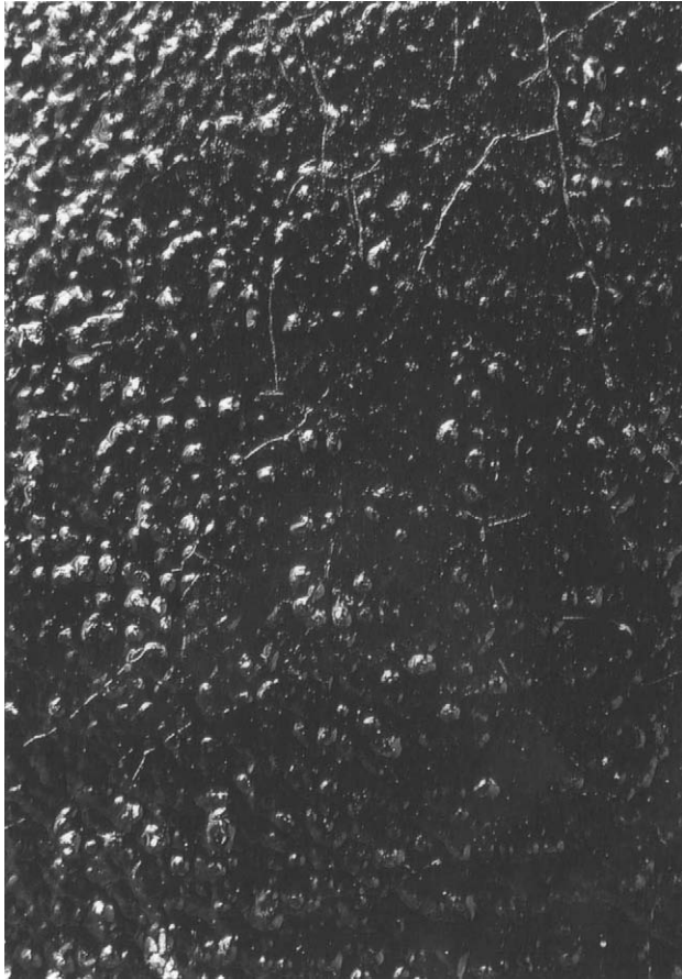
Figure 13. Detail of Madame X , the bodice, which reveals a surface texture of rounded protrusions, the result of the formation of lead fatty acid soaps that have developed in the ground layer as it aged
