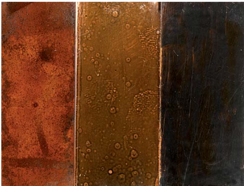
11. Three coupons of stoved varnish containing Burgundy pitch. From left to right: no carbon black, some carbon black, more carbon black
