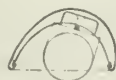
Fig. 2.—Show Case Reflector, 2 in. wide by 2½ in. deep. Type used in Lipman Wolfe & Co., Inc., store.
