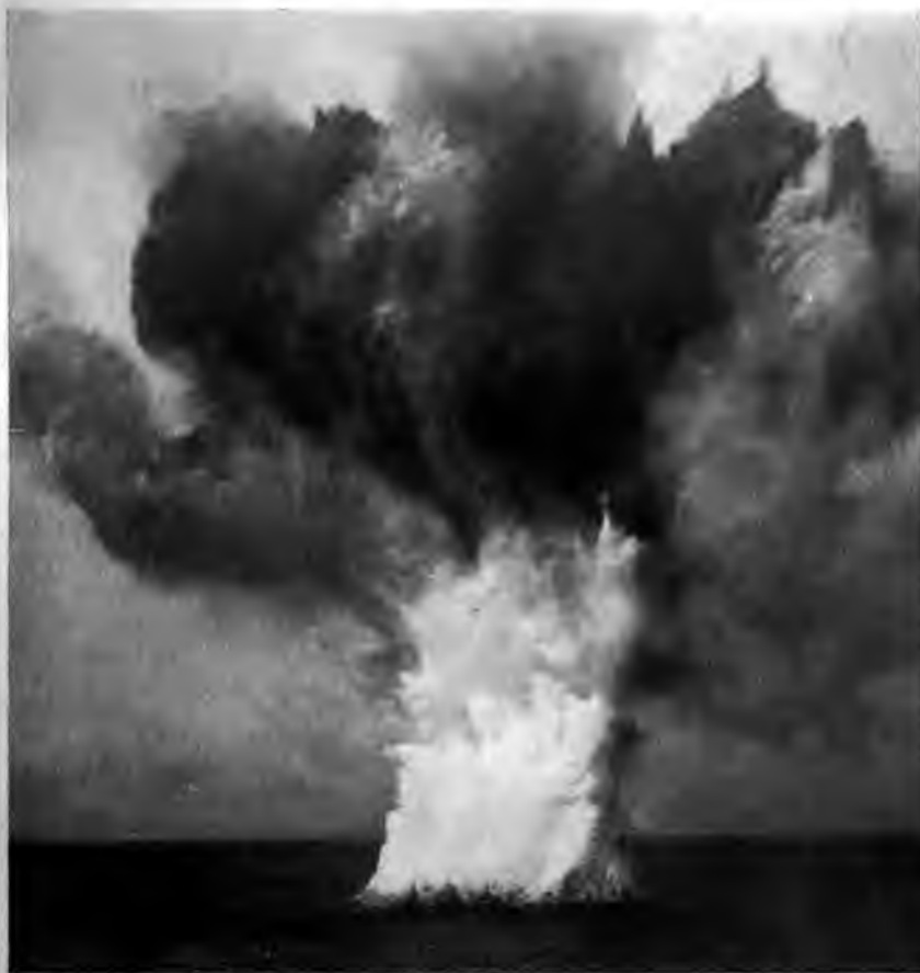
Effect of the Explosion of a 12-Inch Shell Suspended 8 Feet Under Water Sandy Hook Proving Grounds
