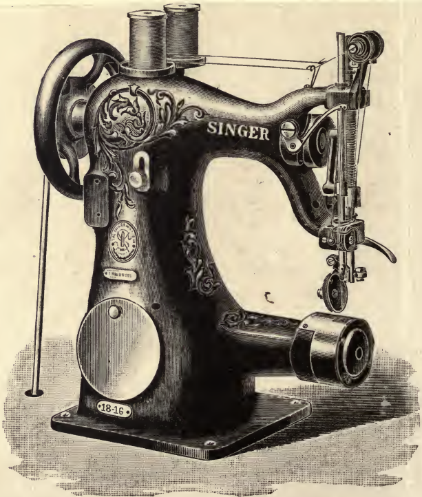
High-Speed Left-Hand Cylinder Machine, with two needles and two shuttles, for making two parallel lines of stitching at one operation. Special adapted for vamping.
