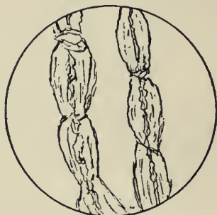
FIG. 45.—COTTON TREATED WITH SCHWEITZER'S REAGENT
