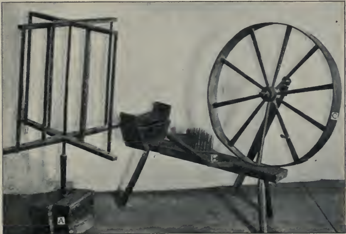
FIG. 31.—A. YARN WINDER B. FLAX HATCHEL C. QUILLING WHEEL FOR FILLING SPOOLS
