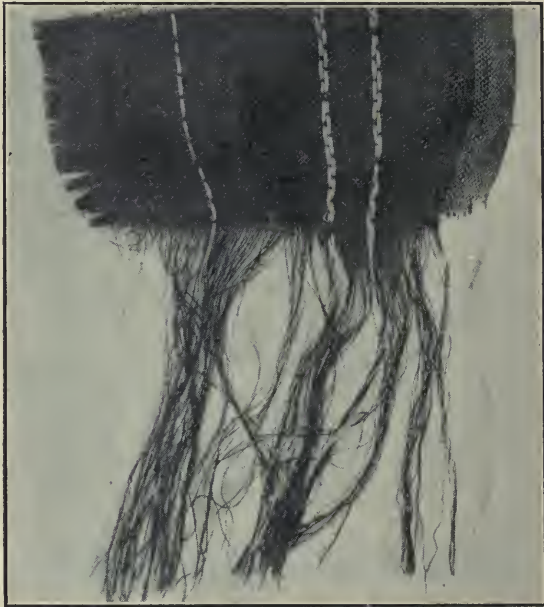
FIG. 37.—MOHAIR, SHOWING COTTON WARP; WOOL REMOVED BY CAUSTIC POTASH
