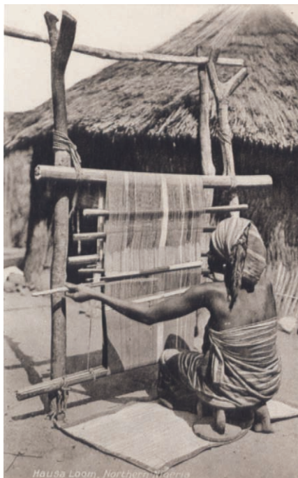
Figure 14. Hausa Loom, Northern Nigeria, early 20th century. Postcard, 5½ x 3½ in. (14 x 8.9 cm). The Metropolitan Museum of Art, New York (PSC 2008.28). A Nigerian woman at work on a single-heddle loom inserts a weaver's sword into the shed—the opening between the odd and even warp yarns—before passing the weft yarn horizontally through the shed.
