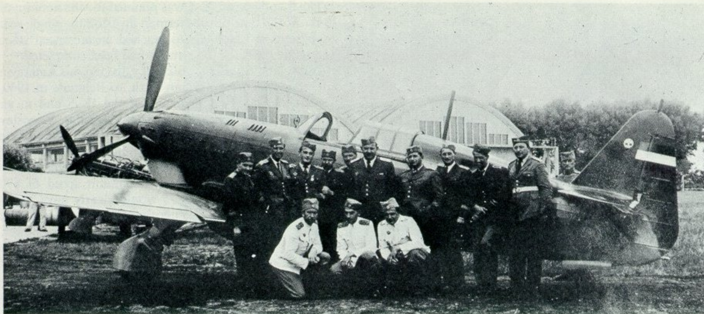
The first-line IK-3 in the summer of 1940. Most apparent revision is the strengthened windshield and cockpit canopy also seen in Photo No. 10 in the earlier photo-page, "IK-3 in close-up". Some of the pilots of this, the 51st Grupa, also appear on the facing page.
