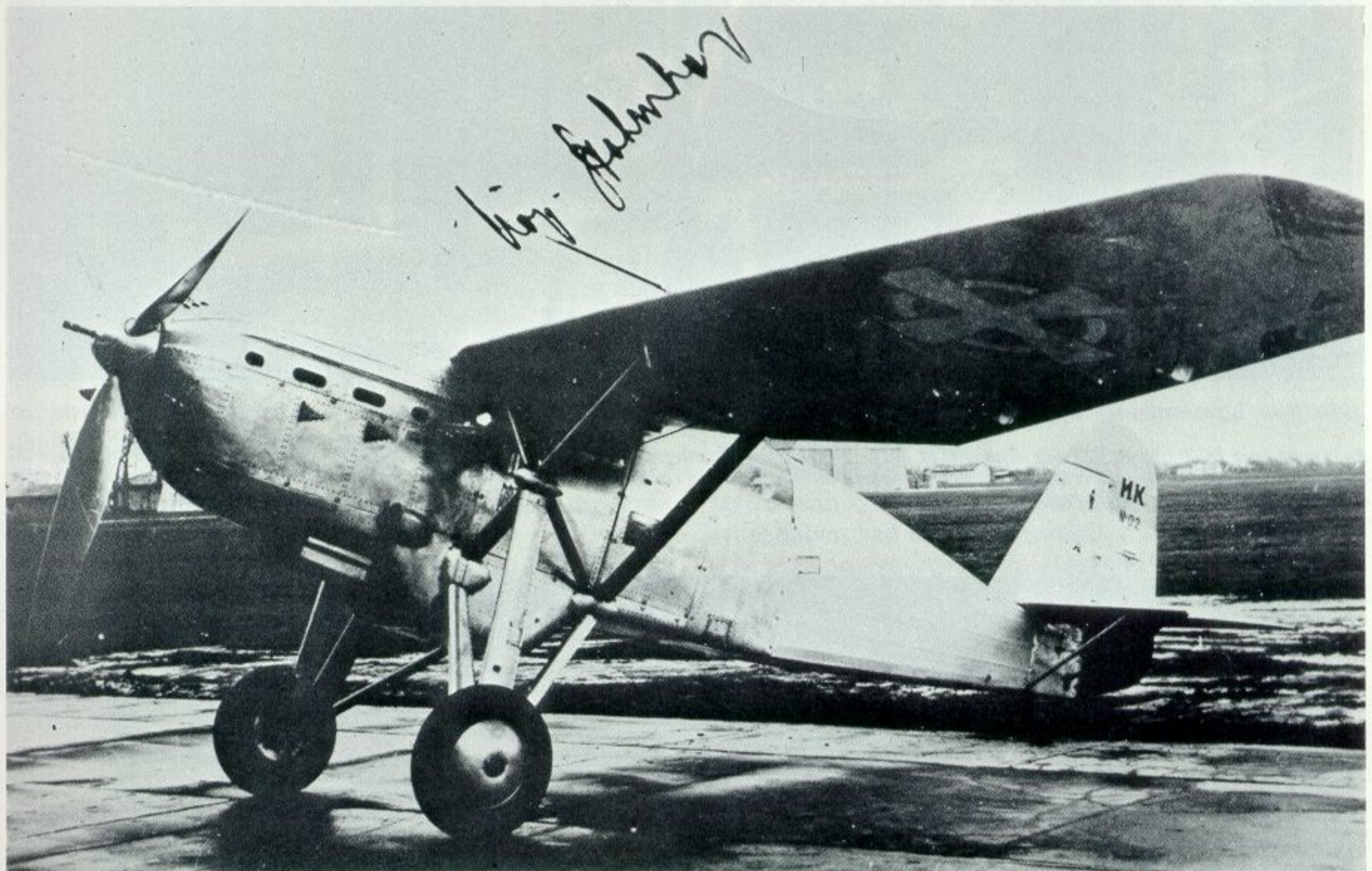
Spring 1938, with traces of snow beyond the hardstanding at Zemun airfield. The second prototype, the IK-02 shows for the first time the hub-firing cannon. The ventral oil cooler is visible because the radiator bath originally incorporating it has been considerably cut back. Test pilot Janko Dobnikar provides the signature as well as these two photographs.
