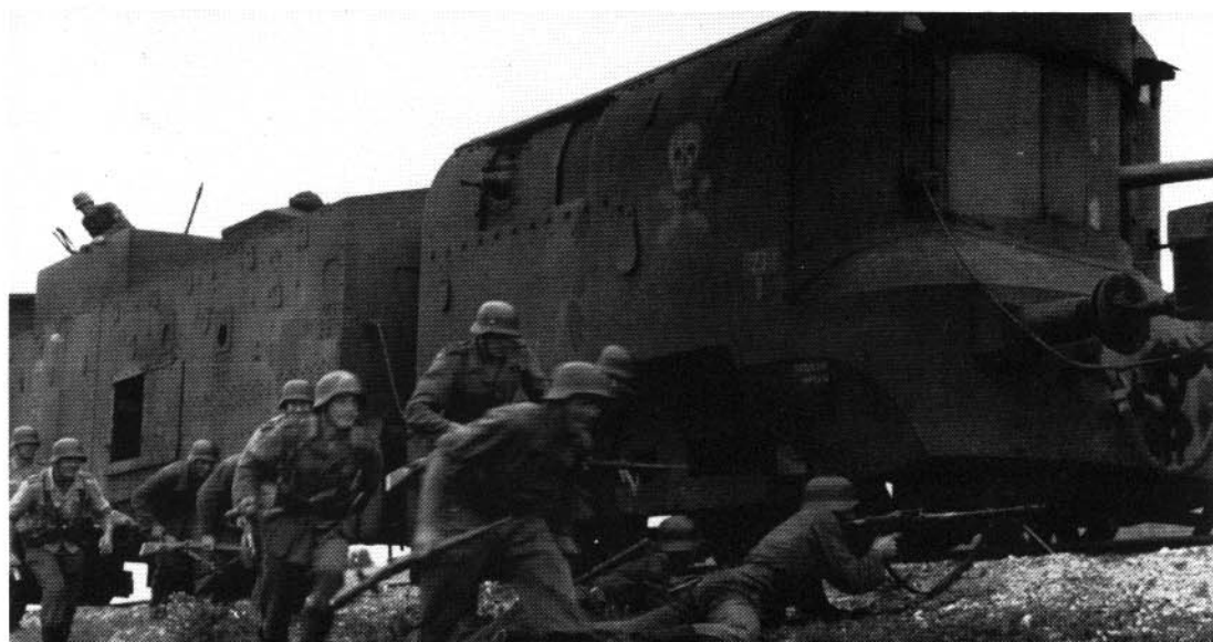
Armored Train No. 23 in service in the Balkans (1941/42). Before and behind the locomotive (No. 93,220) are auxiliary boxcars, but the train also includes armored infantry cars. On the pusher car (far right) is a trolley. While the forward artillery car has a rotating turret, the rear cannon (at left) is still housed in a casemate in a car that comes from an Austro-Hungarian armored train of World War II (probably reaching the Wehrmacht as Czech or Polish booty). (2 x BA)
