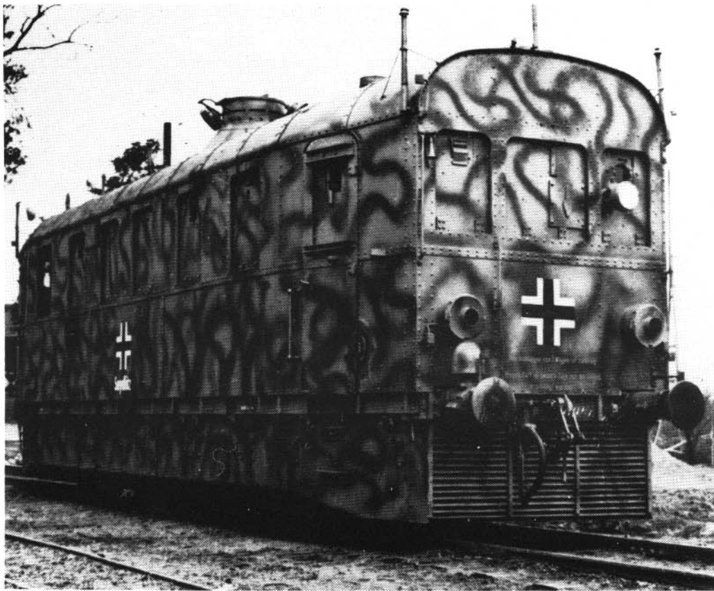
Left: Of the 15 armored railcars built at the beginning of the war, only the last (No. 15), shown in this picture, remained in service after the summer of 1940, and even to the war's end. Its appearance lets one suspect the descent from passenger cars. (BA/MA)
