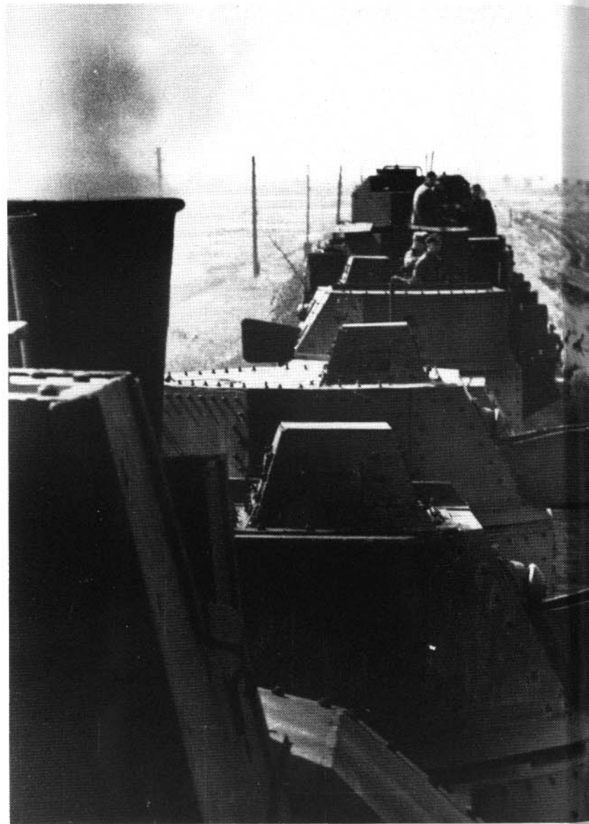
Another broad-gauge armored train made of captured Russian rolling stock. Its being armed with four guns (though by the thickness of their barrels they are smaller than the usual 7.62-cm caliber) shows it to be a regular armored train, perhaps of the reequipped 26-31 series, but a more precise identification based on this pictorial material is impossible for the time being. (3 x BA)
