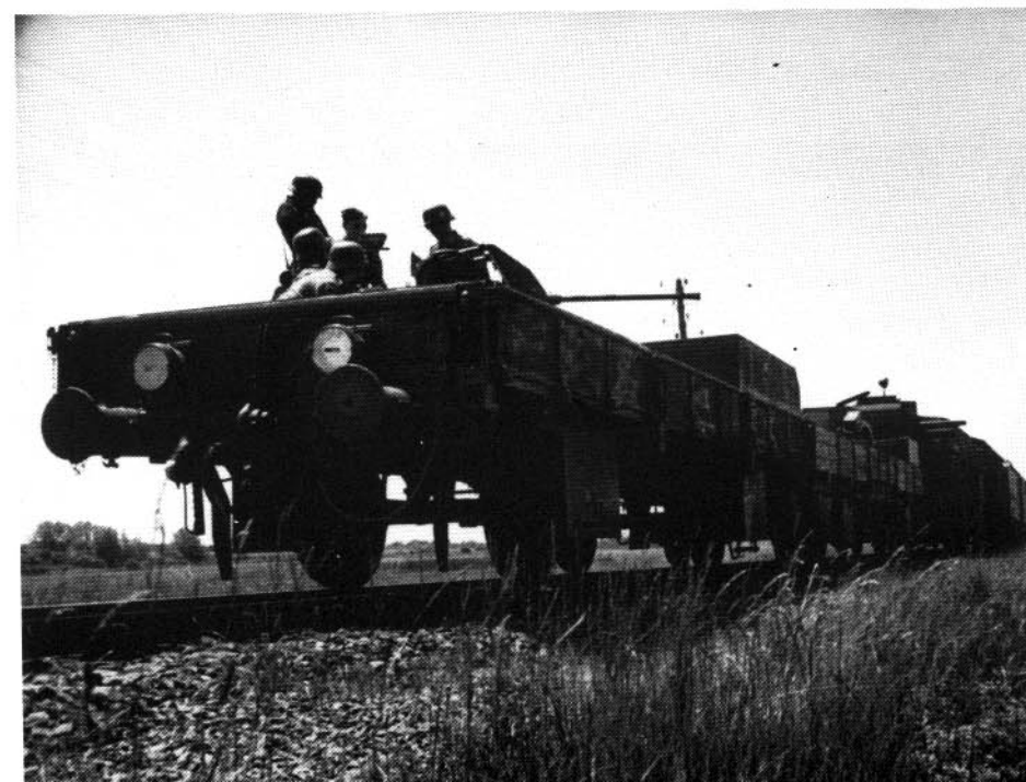
Pictures below: Armored Train No. 22, assembled from captured Polish rolling stock, in France (probably in 1942). Behind the artillery car with its two 7.5-cm guns is another boxcar for the infantry. The right picture shows a 2-cm anti-aircraft gun on the front pusher car (with armored low walls). (2 x BA)
