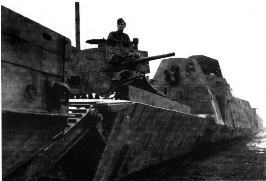
Two pictures of Armored Train No. 63 on duty. At left one can see the loading ramp extending under the pusher car. The second machine gun in the hull of the 38(t) tank has been
