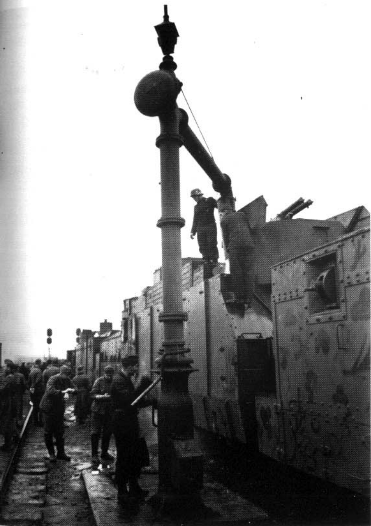
Above: Locomotive maintenance caused a serious problem in Russia, as the coal was of poor quality and the stations with water supplies (as in picture) were rare. (BA)
