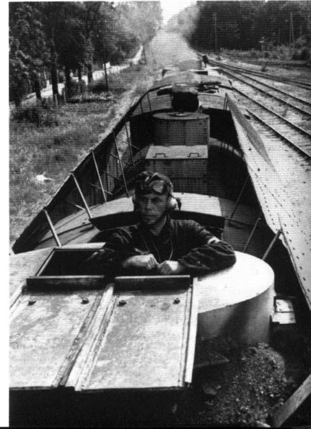
Further details of Armored Train 22. Left: Before the rotating turret of the forward artillery car is a 2-cm anti-aircraft gun on an armored flatcar. Above: Along with the 2-cm anti-aircraft gun, twinned machine guns in sliding roof hatches could also be used for defense against aircraft.
