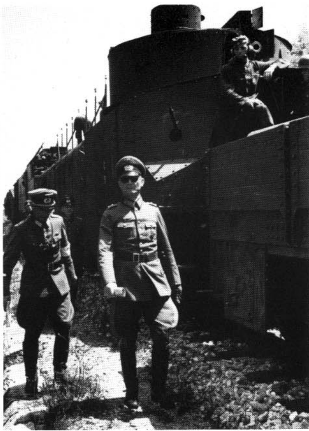
Left: the rear part of Armored Train No. 22, which is being inspected by a commanding general: this artillery car carries only one 7.5-cm gun (note the machine-gun port); in front of it is the command car with the antenna running around the roof. (BA)
